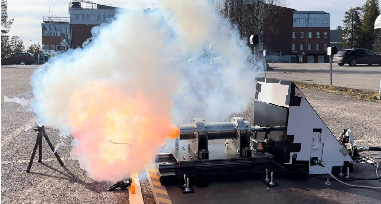
First ignition test of a hybrid rocket propulsion system preparing for a static hot fire test. (Credit: Project RAVEN at the Kiruna Space Campus, LTU, email: kiruna.raven@gmail.com )
